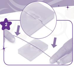
Insert the string into the slots of the shape mold.
