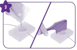
Pour the powder into the mold and remove the exceeding powder with the scraper, leveling it. Place the leftover powder inside the extra bags.
